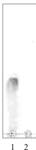
Fig. 4.16 Thin layer chromatography (TLC) of E2-1 fraction of Q. phillyraeoides ethyl acetate extract. Chromatographic fractions were checked by normal-phase thin layer chromatography (silica gel 60 F 254 ) using a mixture of hexane:ethyl acetate:methanol (5:5:2). Purified fraction E2-1 (QPE-2) showed a clear spot.
