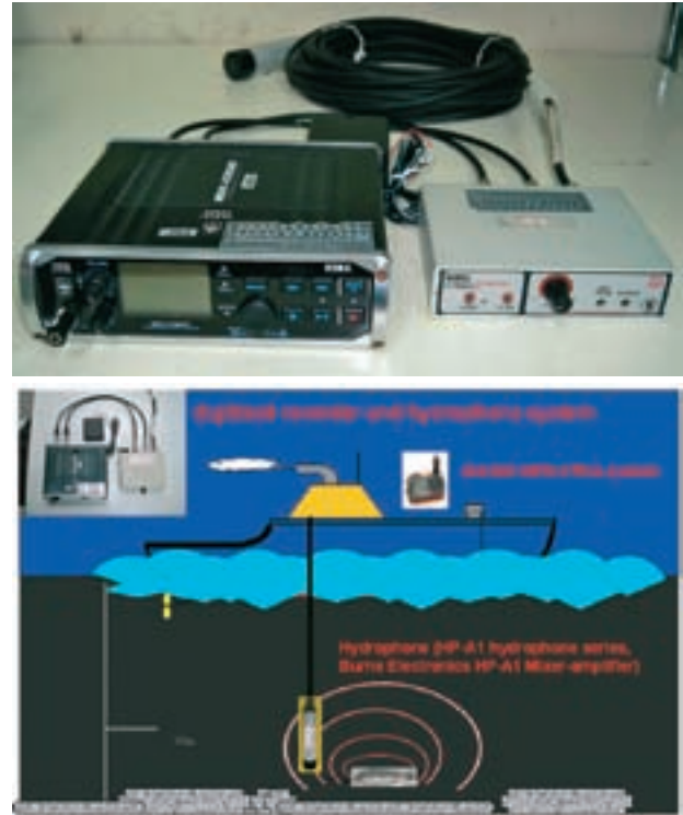
Fig. 1 The sound recording system contains a hydrophone unit (a hydrophone and amplifier) and a digital recorder (Underwater ambient biological noise can be recorded using the portable recording system and the locality of the monitoring stations is recorded using GPS.)
