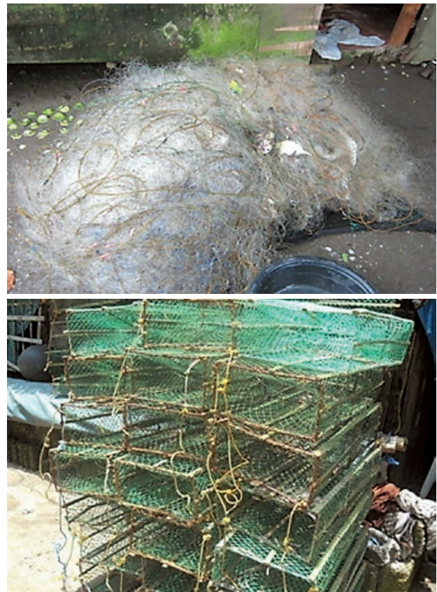
Fig. 6. The most common fishing gears used in crab fishing (Upper: crab gill net, lower: crab pot).
