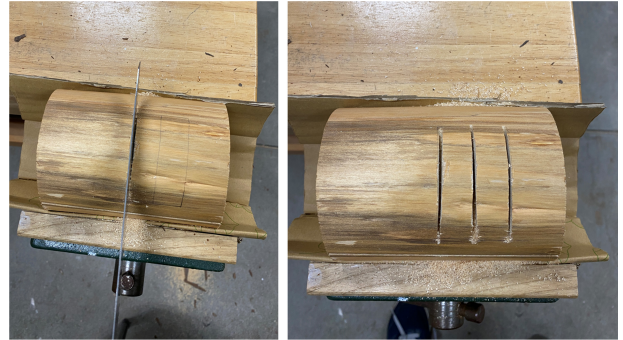
図4. のこぎりによる溝切り (左:加工の様子、右:加工後) Groove cutting by saw (left: during processing, right: after processing)
