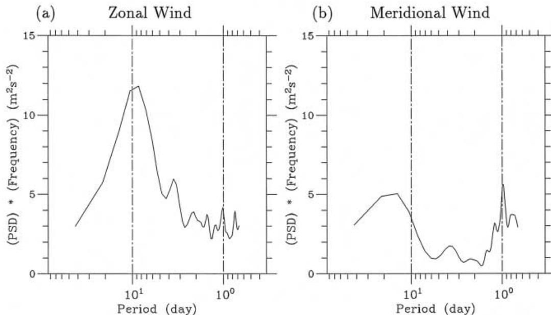
Fig. 5. Spectral analyses of: (a) BLR zonal wind; and, (b) BLR meridional wind averaged for 1–2 km height range. Vertical dashed-and-dotted lines indicate the diurnal oscillation (period of one day) and the 10-day periodicity.
