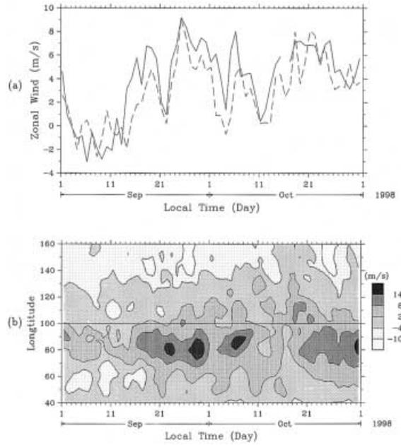
Fig. 9. (a) Time series of zonal winds. Solid curve is BLR wind averaged every 60-min, and over 0–1 km height range. Dotted curve shows NCEP 850 hPa grid point data. (b) Time-longitude cross-section of zonal wind at 850 hPa by NCEP.
