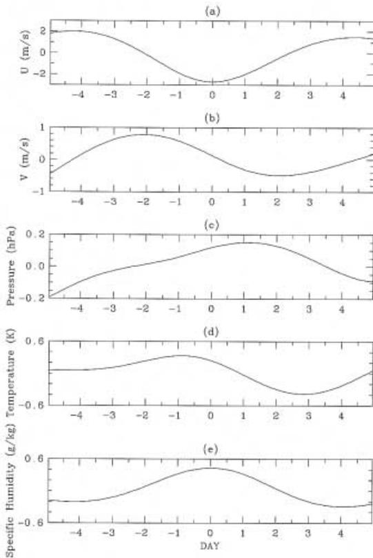
Fig. 8. Composite time series of 7–13 day filtered: (a) zonal wind by BLR averaged over 1–2 km height range; (b) meridional wind by BLR averaged over 1–2 km height range; (c) surface pressure; (d) surface temperature; and, (e) surface specific humidity. The horizontal axis represent day number from westerly wind minimum hour.
