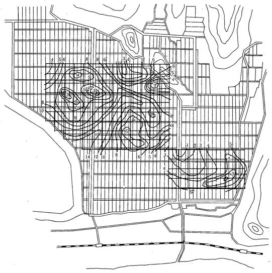
Fig. 4 Result of cone penetration test. (equiconeresistance line)
